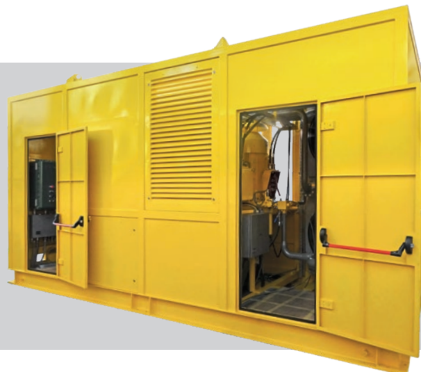
Container with HPU, electric panel and PLC for FPSO marine vessel
